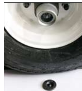
All transportable units have easy lube hubs.
